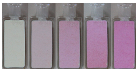
Figure 12. Complex 1-Zn in poloxamer 407 was exposed under different radiant intensity of UV. From left to right: 0, 25, 50, 75, 100 \mu\text{W}/\text{cm}^2 . Exposure time was 2 min.
